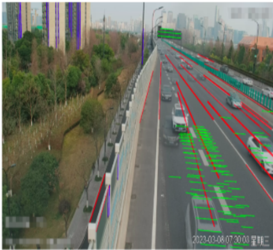
Figure 2. Extract road features to find parallel lines, horizon etc. image adapted from [6]
